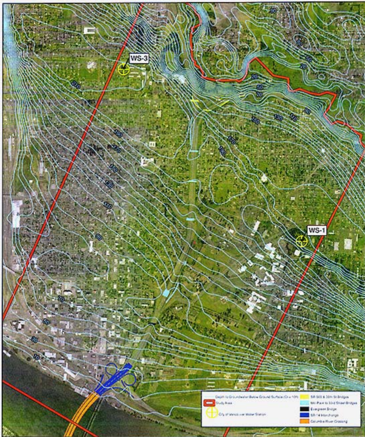
Exhibit 3-9: Depth to Groundwater Level Contour Map May 1995 Troutdale SSA Evaluation
